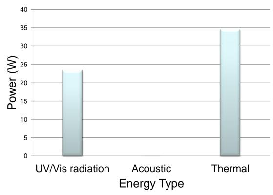
Energy distribution in electrohydraulic spark discharge
